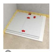
$\dots$  and screw together with the **fermacell** Powerpanel H<sub>2</sub>O Floor Screws, included in the pack (screw spacing approx. 15 cm)
